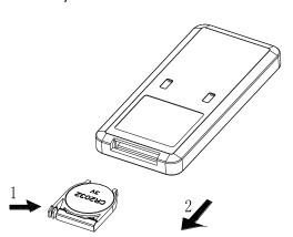
Method for opening the battery cover: firstly, press in the direction shown by arrow 1 to break away the upper buckle of the battery cover, then pull out of it in the direction shown by arrow 2.
