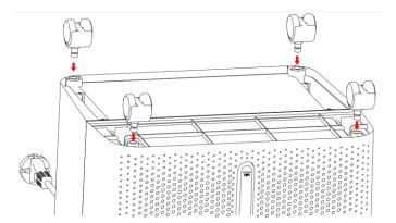
Attachment of the caster rollers may be required. The caster is placed into the hole in the direction of the arrow until the metal end of the caster contacts the plastic end.
