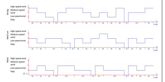
Sleeping wind : Operate at the speed set by the user and reduces the speed according to the preset rules. This mode prevents people from physical discomfort due to high speed wind during sleeping. Rules for wind operation in the natural wind mode are as follows:
