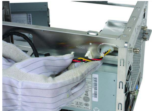
② Feed the HDD cable through the reverse hole as shown and attach to storage devices.
