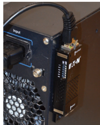
Eaton EMP Gen 2 installed
