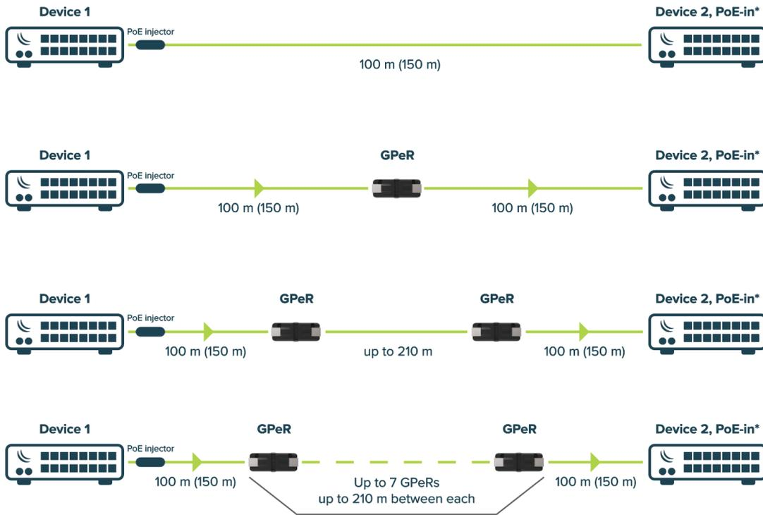
\* Voltage drop on the cable and on GPeR units needs to be taken into account when calculating PoE-in possibility, in case of insufficient power take off PoE jumpers to disable Passive PoE passthrough and use other power source for Device 2.
