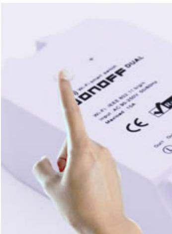
2. Press the pairing button for 7 seconds until the green LED blinks like below: the LED blinks 3 times and on repeatedly
